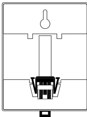
The EWS 102 can be mounted either on a DIN rail or on a flat surface using a single screw mounting aperture in the rear plate.
