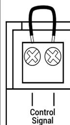
If required, wire the control signal input to receive a suitable signal indicating the car has stopped at the landing with the doors opening or closing, for example the brake open close circuit.
