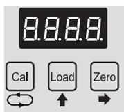
Multi Analog version only: See note 3 page 1. After the EWS 102 calibration and setup has been completed, place the the lift at the lowest floor level and rezero following the process on page 2, this will finalise the Analog output calibration.
