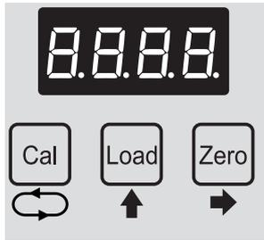
To begin the system setup press the **Cal** and **Load** buttons together
