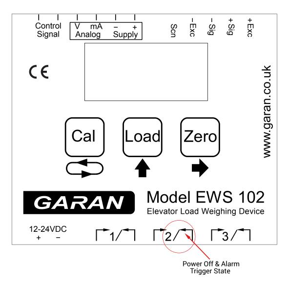
As the EWS 102 is a safety device, the label shows the default position of the relays when no power is being applied to the unit. When power is applied the relay switches state.
