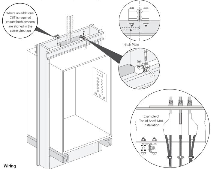
Once the CBT sensor has been fitted to the beam, terminate the cable at the EWS 102 Elevator Load Weighing Device , if during calibration the weighs backwards, swop the red and white signal wires.
