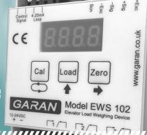
Our EWS Control Unit provides a simple yet powerful range of load weighing options. They work with a variety of sensors and can be easily configured using our straightforward, step by step, set up procedure. Calibration is simple and can be achieved with either a known or full load.
